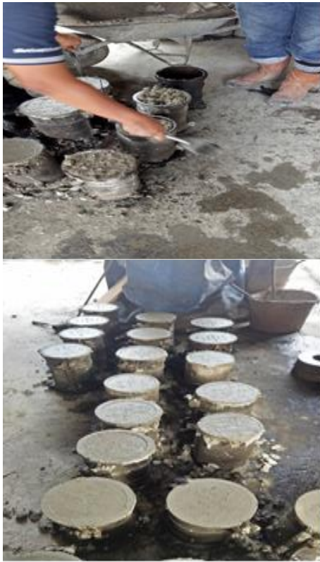
Fig. 1 Concrete sample testing.
